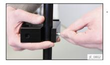
Insert the rod in the groove in the stand support so that the rubber end of the bar is oriented upwards and secure the bar with a screw.
