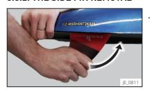
To remove the fin, grasp the fin and pull upwards.
