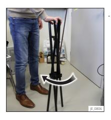
Gently turn clockwise the ends of the rods which are most distant from the clamp of the stand.
