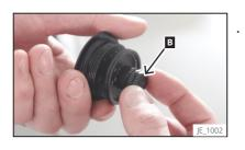
Remove the balancing valve **B** , with your hand by turning it anticlockwise.
