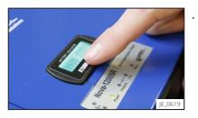
By touching the bottom part of the display, you can change the type of the information shown on the charger display.
