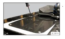
Remove 4 (four) socket head screws from the motor cover.
