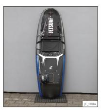
Place the board vertically and let the water drain out of the motorized surf.
