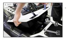
Place the battery pack in the Jetsurf Electric so that the battery plug **B** and battery socket **a** are against each other (see the figure *JE\_0605*).
