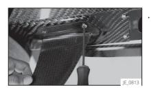
Insert the removed screws in the openings on the main fin and tighten the fin.
