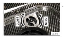
Remove the cover of the ventilation system A by turning it anticlockwise.
