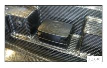
• Put the battery connector cover on (P014145).
