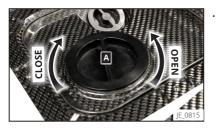
Remove the inspection cover (A) by turning it anticlockwise.
