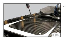
Remove 4 (four) socket head screws on the motor cover.
