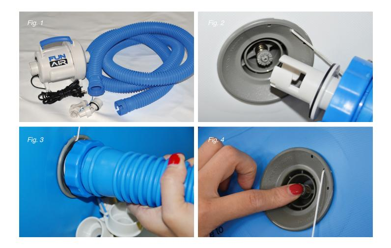
During inflation, ensure the air valve is in the closed position by pushing on the stem to see it if depresses about 1/4 inch (FIG. 4). If it does not depress 1/4 of an inch, then rotate the stem 1/4 turn left, and it should pop out to a shut position. The valve is now closed. If the valve is open during inflation, then it will release air from the tube when the pump is removed.
